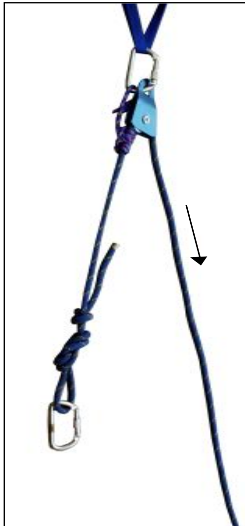
1:1 Pulley system w/self-minding ratchet
